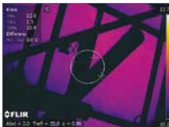
Inspection from the back shows no hot spots, the hot spots in the previous thermal image taken from the front were caused by cloud reflection.
